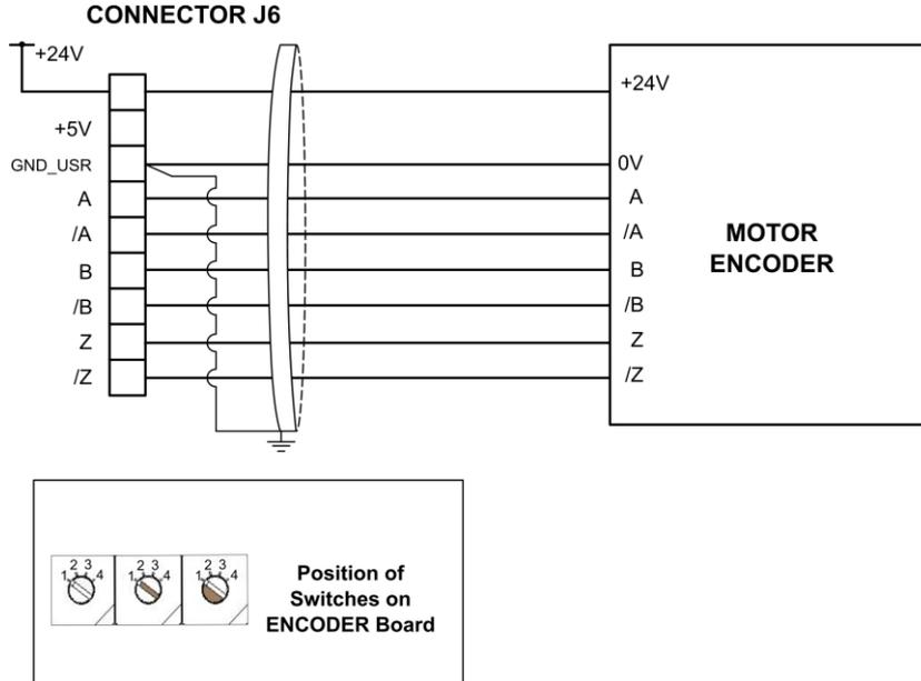
**Note:** Ground connection using shielded cable on the drive side only.
