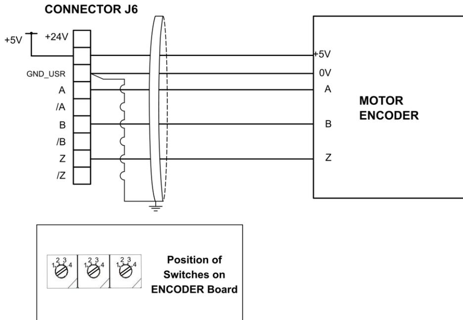
**Note:** Ground connection using shielded cable on the drive side only.
